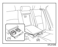
The cup holder (1) for rear seat passengers is extended ready for use when the armrest is tilted down and the button (2) is pressed. Push the cup holder backward to store it.
